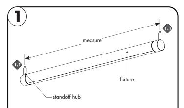
Note: Two junction boxes are required for this installation. One at each end of the fixture.
